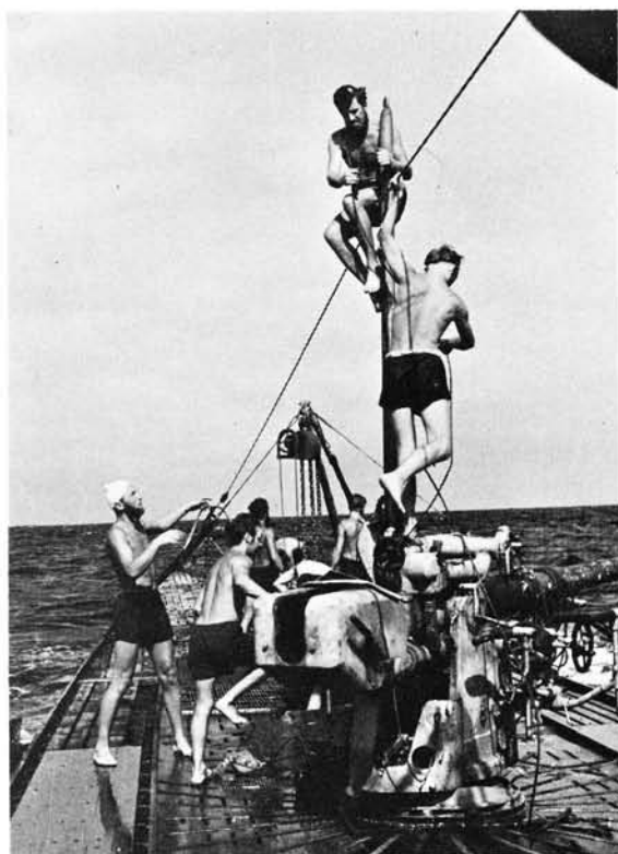
The transfer of on-deck torpedoes was hard work. Booms and cranes had to be set up and firmly lashed, so that with the help of blocks and tackles the heavy torpedoes could be lowered through the narrow, sloping hatch into the fore-ends, even when the boat was rolling in a swell
