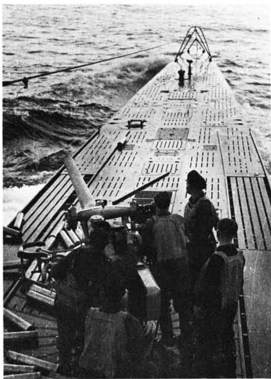
When the first torpedo did not have sufficient effect and other torpedoes had to be economised, the 10.5cm gun came into action, as seen here against the Eskdene. On the foredeck, aft of the jumping-wire, the T-shaped head of the underwater sound location device can be recognised (Bundesarchiv)
