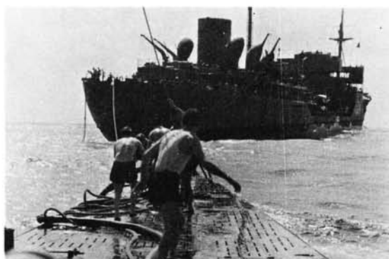
On 5 May 1941, in mid-Atlantic, U-107 met the supply-ship Nordmark, sister-ship of the famous Altmark, to replenish fuel. The towing-hawser and the fire-hoses for taking on fuel are prepared (Bundesarchiv)
