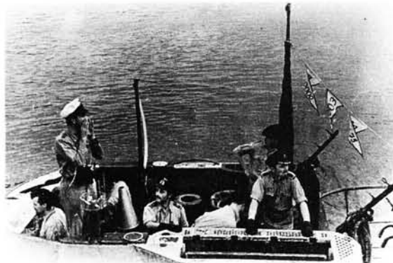
Bridge of a U-boat, 1943: Aft of the Captain, the opening for the LW-DF aerial (also MW); immediately behind the opening for rod-aerial. Aerial-target periscope retracted (middle opening); surface-target periscope raised. Behind, 2 MG 151. In front, opening for the retracted 'Hohentwiel' radar aerial (upper side of the beam aerial recognisable). Left of the Captain, round dipole aerial of the 'Naxos' radio-location apparatus From 1943, the bridge of U-107 was similar (BfZ/Gröner)
